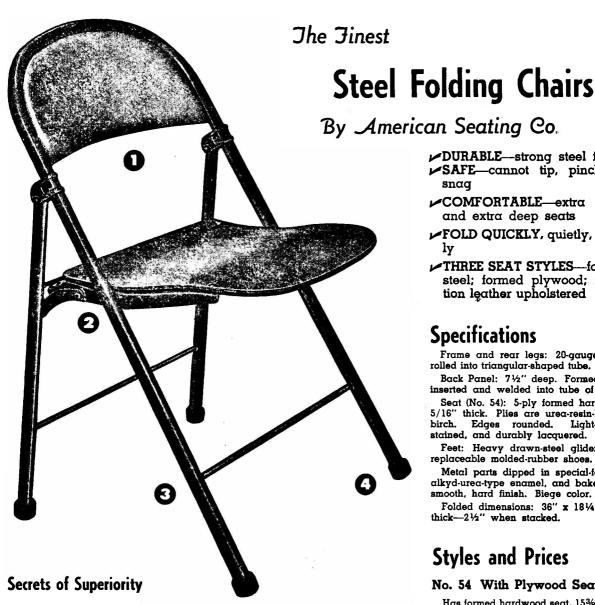
1. Back panel is dieformed from one piece of steel, inserted and welded into the tubing. Bottom edge is rolled for rigidity and smoothness.
